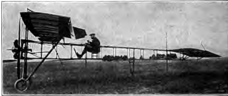
Fig. 54. Henri Farman in His New Monoplane. The Frame is of Steel-Tube Construction
